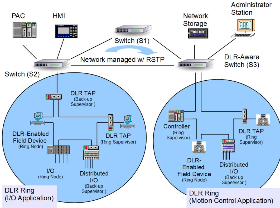
**Figure 2 - DLR Network with two non-overlapping rings**
