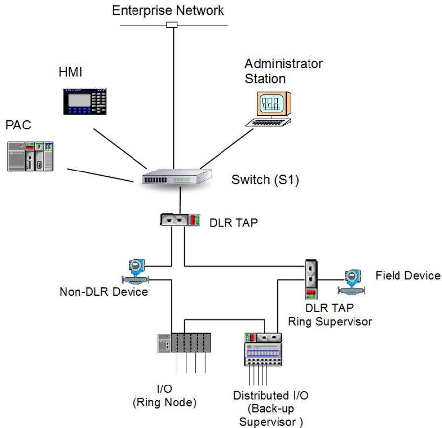
**Figure 3 - DLR ring with a Non-DLR Device**
