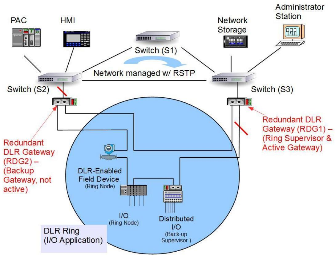
**Figure 8 - DLR ring with 2 Redundant Gateways**
