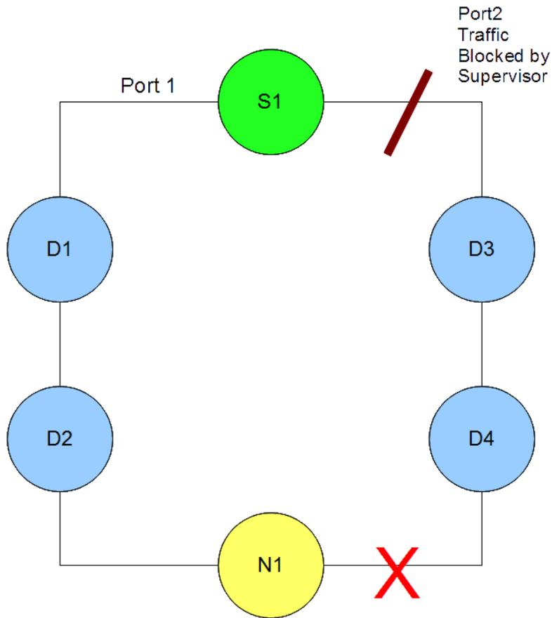
**Figure 4 - Simple ring with one Non-DLR node**
