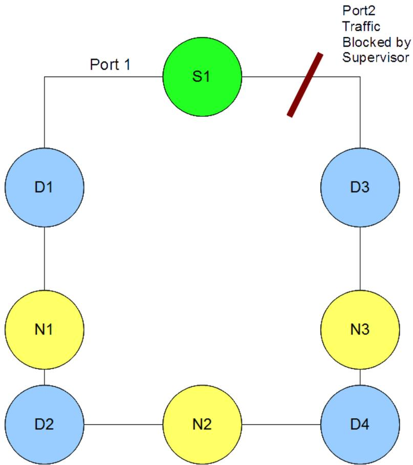
**Figure 6 - Simple ring with three Non-DLR nodes interspaced**
