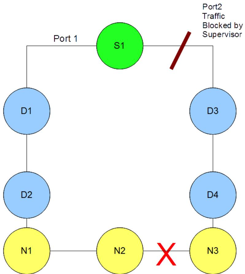
**Figure 5 - Simple ring with three Non-DLR nodes**
